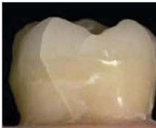
Figure 4: Fractured RNC specimen without fragment.
