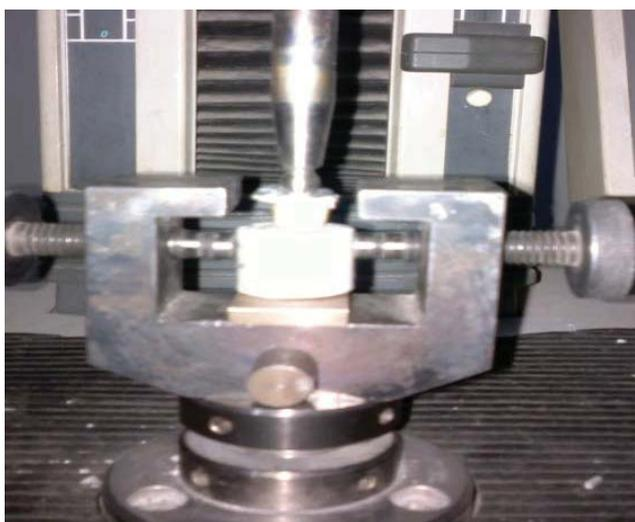
Figure 2: Fracture test of specimen.
