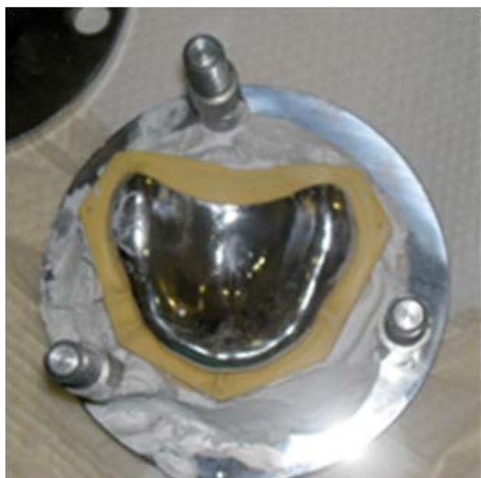
Figure 5: Model fixation in the dental reline jig and placing the corresponding matrix.
