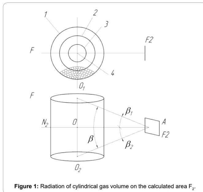
Figure 1: Radiation of cylindrical gas volume on the calculated area  $F_2$ .
