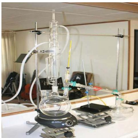
Figure 1: Soxhlet apparatus.
