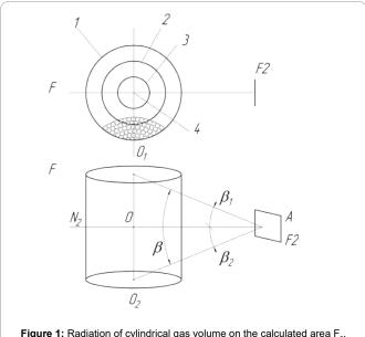
Figure 1: Radiation of cylindrical gas volume on the calculated area F<sub>2</sub>.
